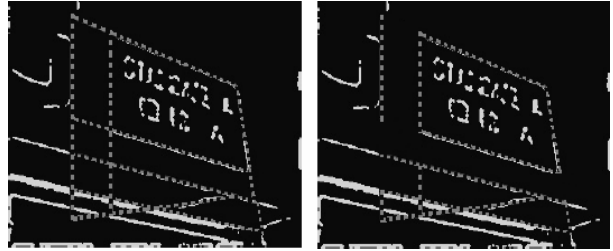
Figure 3. Checking possible segments that form the boundary of a signboard. Left: impossible segments are removed. Right: segments are remained after density checking.
