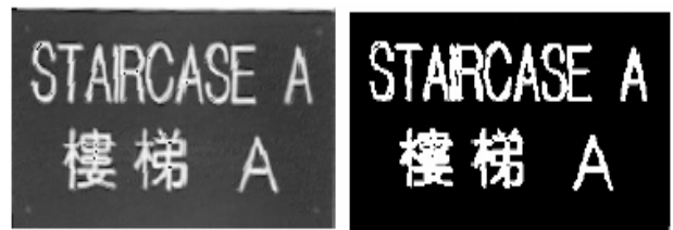
Figure 10. Result after thresholding
