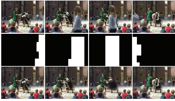
Figure 3: Some results on the “performance” video. The three rows show the original frames, the manually removed regions, and the video completion results by our algorithm, respectively.
