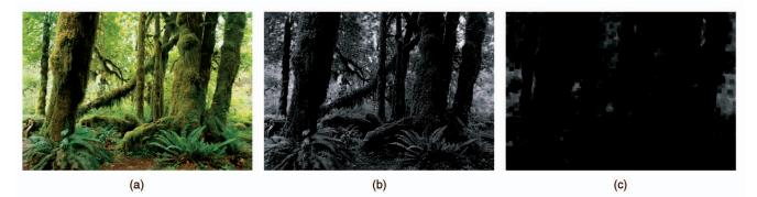
Fig. 3. Calculation of a dark channel. (a) An arbitrary image J. (b) For each pixel, we calculate the minimum of its (r, g, b) values. (c) A minimum filter is performed on (b). This is the dark channel of J. The image size is  $800 \times 551$ , and the patch size of  $\Omega$  is  $15 \times 15$ .
