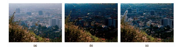
Fig. 10. (a) A  $600 \times 400$  hazy image and the recovered scene radiance using (b)  $3 \times 3$  and (c)  $15 \times 15$  patches, respectively (without soft matting). The recovered scene radiance is oversaturated for a small patch size, while it contains apparent halos for a large patch size.
