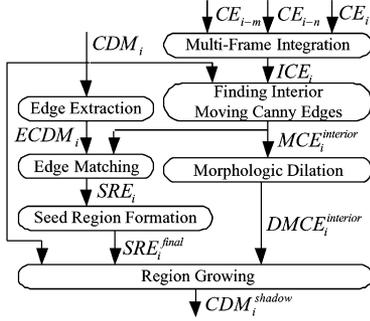
Fig. 4. Block diagram of the shadow region detection.
