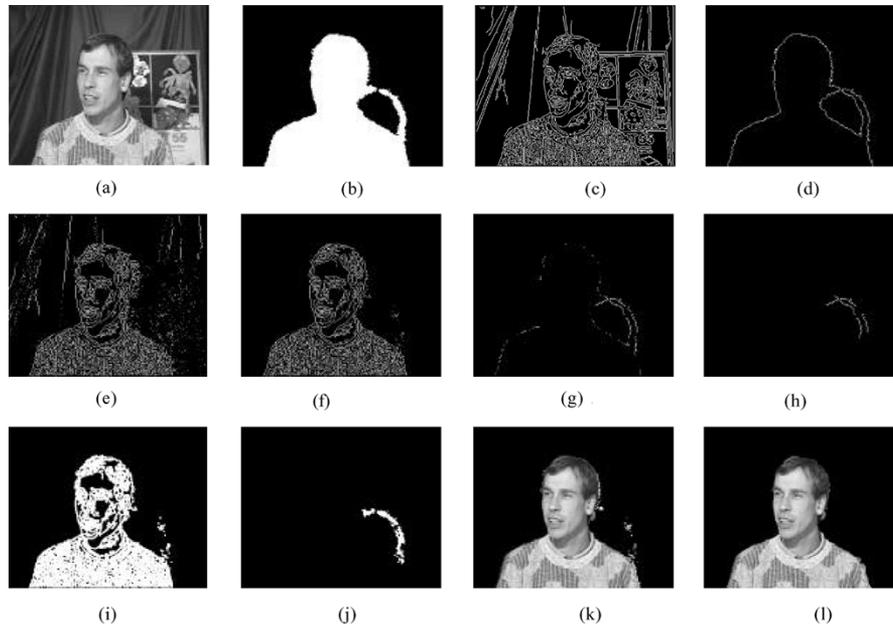
Fig. 2. Illustration of the results of the main steps in our algorithm with frame 46 of the video sequence Erik. (a)  $f_{46}$  of Erik. (b)  $CMD_{46}$ . (c)  $CE_{46}$ . (d)  $ECMD_{46}$ . (e)  $ICE_{46}$ . (f)  $MCE_{46}^{interior}$ . (g)  $SRE_{46}$ . (h)  $SRE_{46}^{final}$ . (i)  $DMCE_{46}^{interior}$ . (j)  $CMD_{46}^{shadow}$ . (k)  $MO_{46}^{initial}$ . (l)  $MO_{46}^{final}$ .
