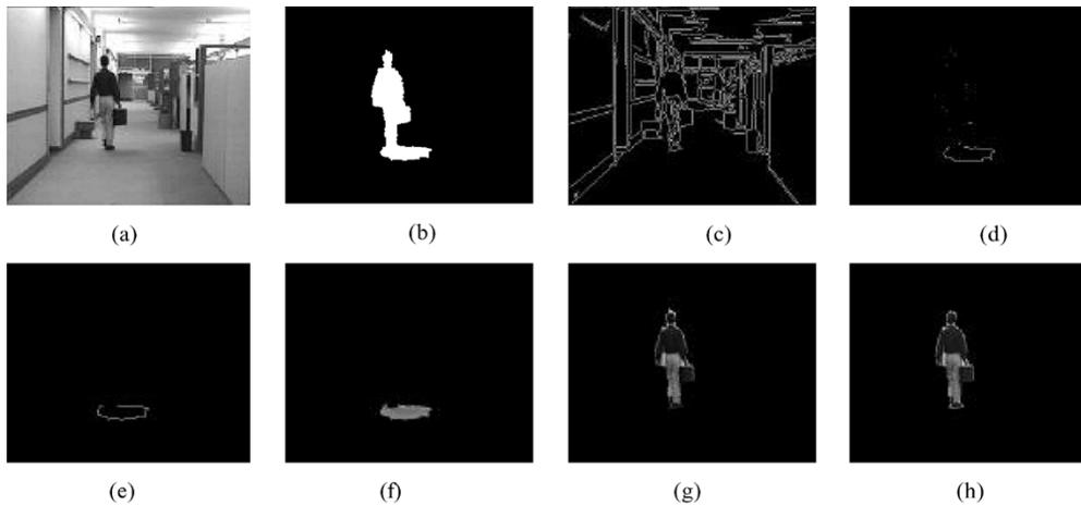
Fig. 3. Main results for the frame 53 of the video sequence Hall. (a)  $f_{53}$  of Hall. (b)  $CMD_{53}$ . (c)  $CE_{53}$ . (d)  $SRE_{53}$ . (e)  $SRE_{53}^{final}$ . (f)  $CDM_{53}^{shadow}$ . (g)  $MO_{53}^{initial}$ . (h)  $MO_{53}^{final}$ .
