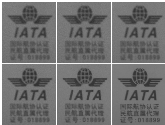
Figure 8. The SR results from eight LR images. From left to right, the top row is direct up-sampling, bicubic interpolation and the IBP result with PSF 1.5. The bottom row is the IBP result with ground truth PSF 2.5, our result and the original HR image.
