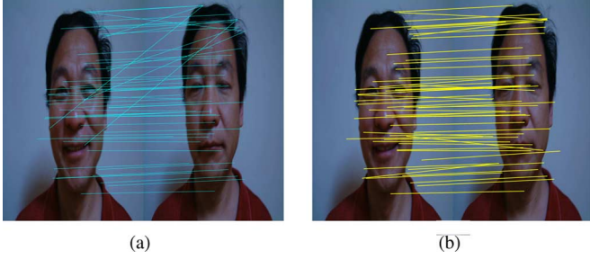
Fig. 4. Demonstration of facial image matching. (a) SIFT feature matching proposed in [17] with threshold t = 0.86 . (b) Better matching result by the proposed RCP algorithm, in which a small threshold t = 0.6 in [17] is used to elicit the robust correspondences for propagation. In both images, 60 matches are produced.
