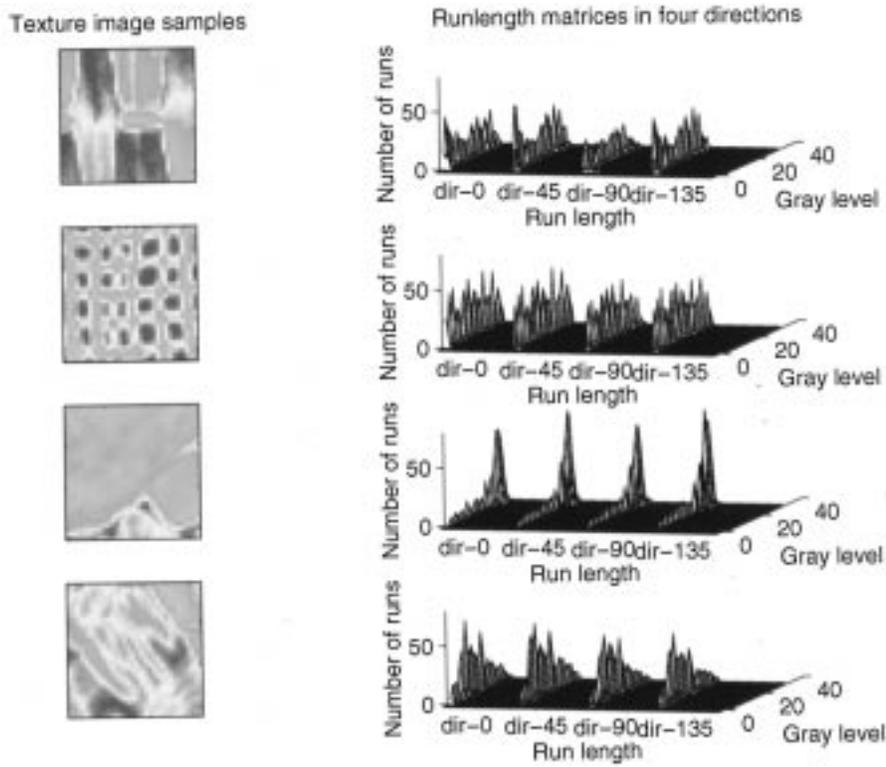
Fig. 1. Four directional run-length matrices of several Brodatz texture samples. Each image sample is of size  $32 \times 32$  with 32 gray levels. The four directional ( $0^\circ$ ,  $45^\circ$ ,  $90^\circ$ , and  $135^\circ$  directions) run-length matrices are combined into a single matrix. The left-most column of each directional matrix is the run-length-one vector, which has much larger values than the other columns.
