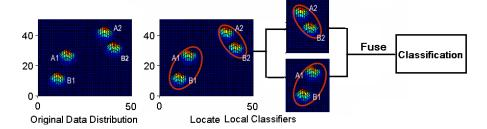
Figure 1. Schematic diagram for designing an ensemble of locally adaptive classifiers. In this example, the data distributions of classes A and B are both Gaussian mixtures (A1, A2 are the two mixture components for class A, while B1, B2 are those for class B). The two ellipses show the locations of the local classifiers.
