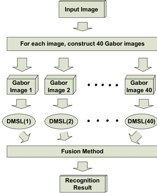
Figure 1. DMSL-based Multi-classifier Fusion Framework on Gabor Images
