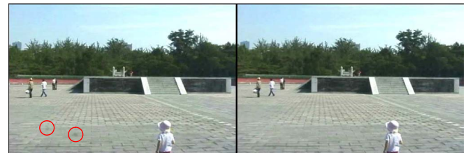
Figure 11: Sensor dust removal. Left: Spots on the camera lens are visible in the original video. Right: The spots are removed from the entire sequence by masking out the spot areas and applying our video completion method.
