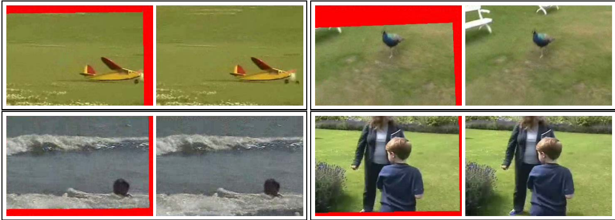
Figure 10: Result of video completion over different types of scenes. In each pair, left image is the stabilized image with missing image area (filled in by red), and right image is the completion result.
