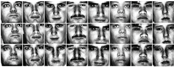
Fig. 3. Demonstration of misalignment (translations) estimation and image reconstruction on the CMU PIE database. Original samples are displayed in the first row, the second row is the corresponding samples with random translations of 4 pixels, and the bottom row contains the reconstructed samples by our algorithm.
